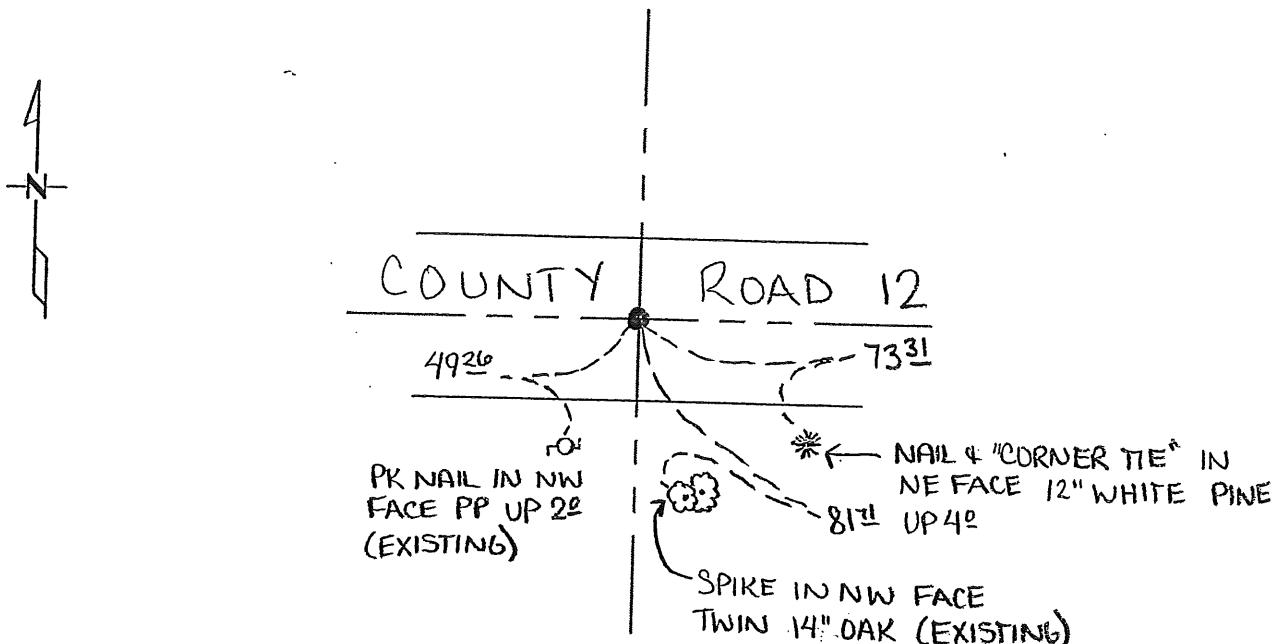
Ties that are found and in good condition are noted as 'existing'. New tree and power pole ties are to the head of a nail with a brass disk marked "Corner Tie".
